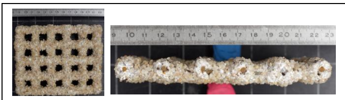
Fig.1: Geocorail's sample after 5 months (Top view on the left, cross section on the right)
