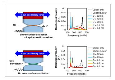
Fig.1 Schematic representation (left) and data (right) of RSM of confined lubricants. While mineral oils solidified under nano-confinement (upper), surfactant-containing oils did not (lower).
