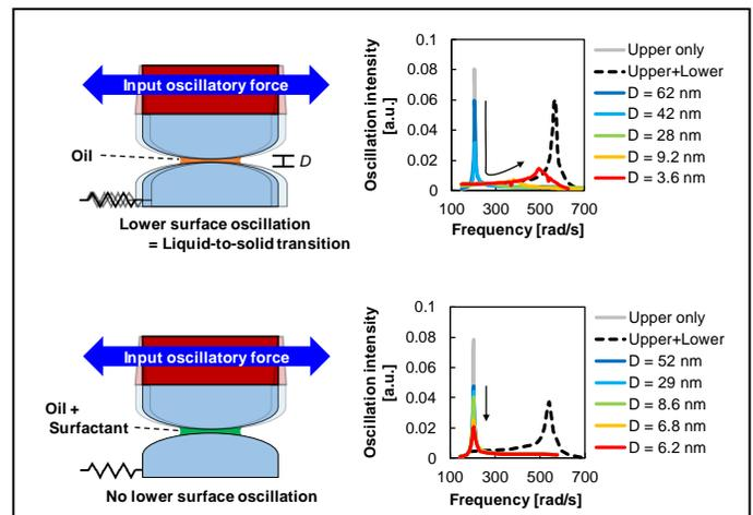
Fig.1 Schematic representation (left) and data (right) of RSM of confined lubricants. While mineral oils solidified under nano-confinement (upper), surfactant-containing oils did not (lower).
