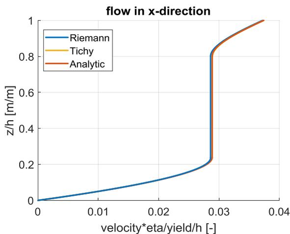
Figure 1 : Typical flow field in x-direction for a Bingham fluid with the use of different methods.
