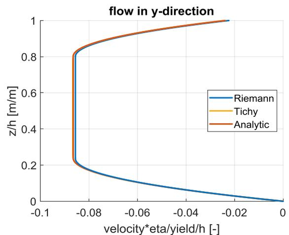
Figure 2 Typical flow field in y-direction for a Bingham fluid with the use of different methods.
