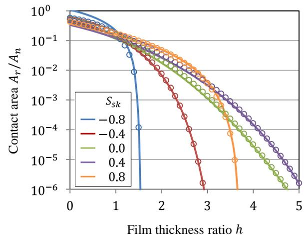
Fig.2 Contact areas under plastic deformation for different skewness (lines: present model, points: theoretical solutions)
