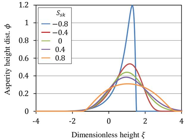
Fig.1 Asperity height distributions for different skewness
