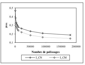
Fig.1 Evolution of the skid resistance versus the number of polishing cycles and load
